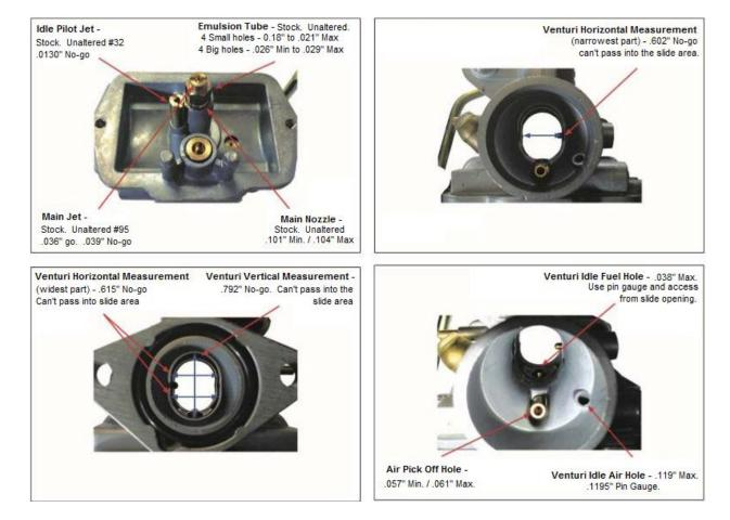
• <u>Carburetor (Continued)</u>: The B&S stock carburetor part #555658 is the only carburetor permitted. No alterations allowed unless stated on this page below. All parts will be
